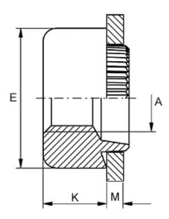
Female thread A = M3Height K = 3.0Outer diameter E = 8.0Plate thickness = 4.7 to 4.9
